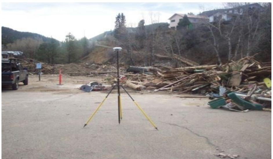
CompassData provided ground control to verify the accuracy of LiDAR data collected to analyze the severity of the floods.
