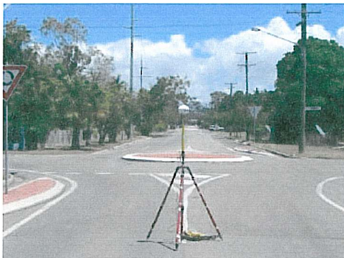
A GPS unit set up on a photo-identifiable point in a road.
